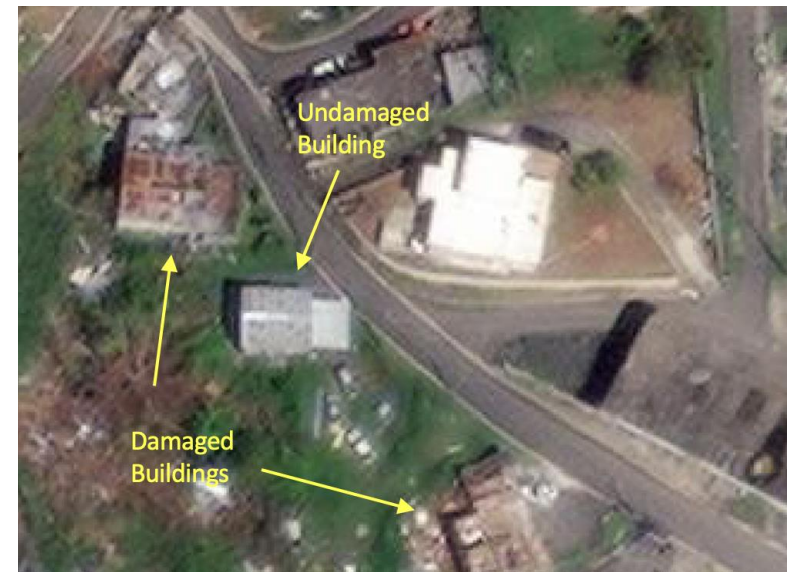
Figure 6: Maxar's GEO-1 satellite data (30-cm resolution) allows the detection of damaged and undamaged buildings from space. This example visual panchromatic product is from October 12, 2017, about one month after the storm had passed. Credit: Maxar Open Data Program.
