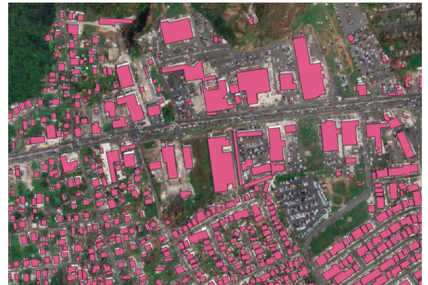
Figure 8. A building footprint map can quickly identify regions where there is a mix of residential (smaller) and commercial (larger) buildings to support labeling of training data. In the image here, it is easy to see the uniform and smaller residential buildings on the bottom half of the image and the larger and non-uniform commercial buildings in the top half of the image. Credit: Bing Maps ( https://github.com/microsoft/GlobalMLBuildingFootprints )
